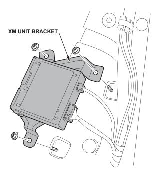
7. Slide the transceiver onto the bracket.
