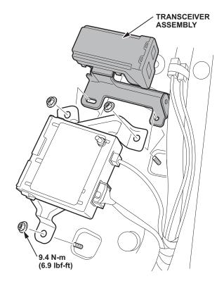
10. Reinstall the XM unit using the three nuts and torque to 9.4 N•m (6.9 lbf-ft).
